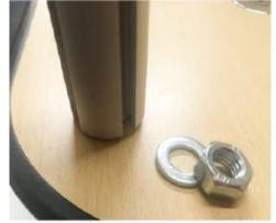
Step 2 Thread the end of the pole through the washer and drilled hole within the desktop.
